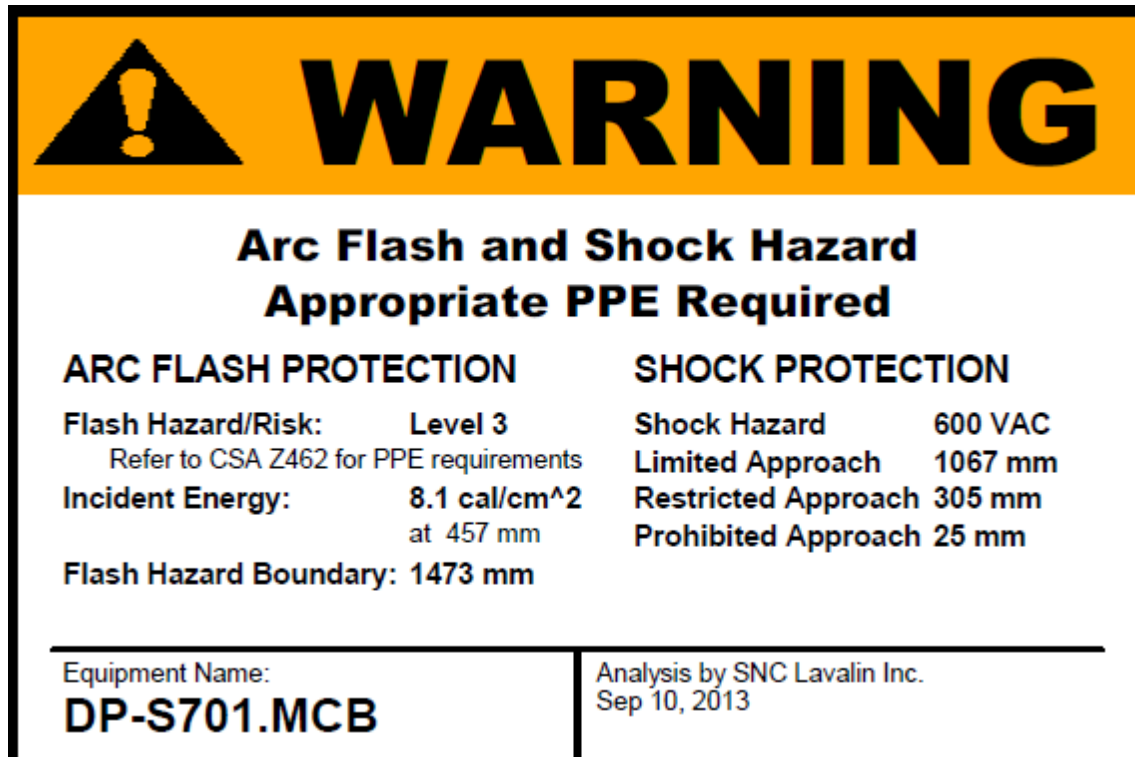
Figure 12-2 : Arc Flash Warning Label, Category 0 through 4 - Large
